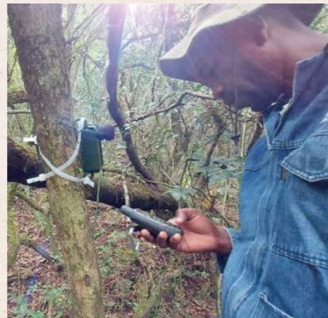
Top and bottom: Installing an acoustic recording unit and marking the GPS location. All photos © Wild Bird Trust
